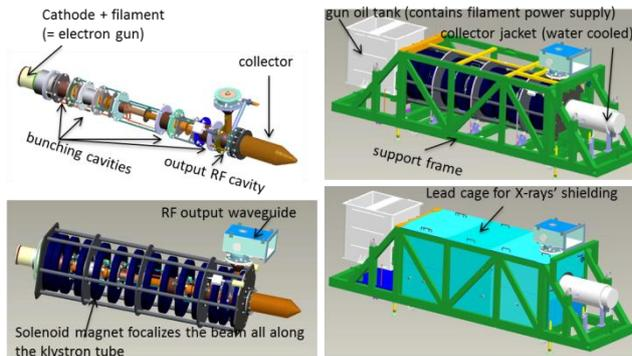
Fig. 5: Different views of a klystron rated for 704MHz / 1.6MW during assembling.
