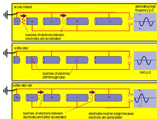
Fig. 3: Principle of linear acceleration in modern particle accelerators.
