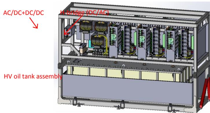
Fig. 8: 660kVA ESS/LTH klystron modulator layout
