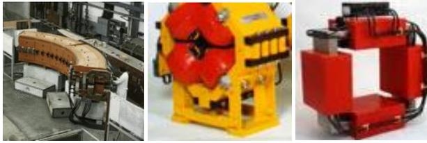
Fig. 6: Different types of electromagnets (left: dipole; centre: quadrupole; right: corrector)
